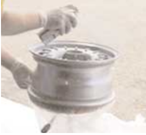
Several thin coats of Wheel Paint & Clear Lacquer are better than a thick one.
