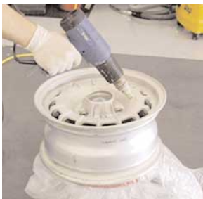
You can help dry and cure the paint by using 75 to 80 degree heat.
